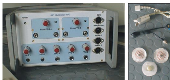
Fig. 1. Multi sensor measuring system capable of simultaneously reading multiple PPG channels, ECG and breathing signals.
